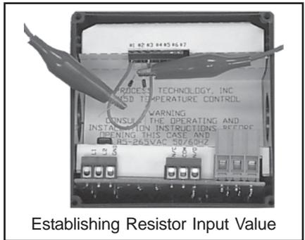
Establishing Resistor Input Value
